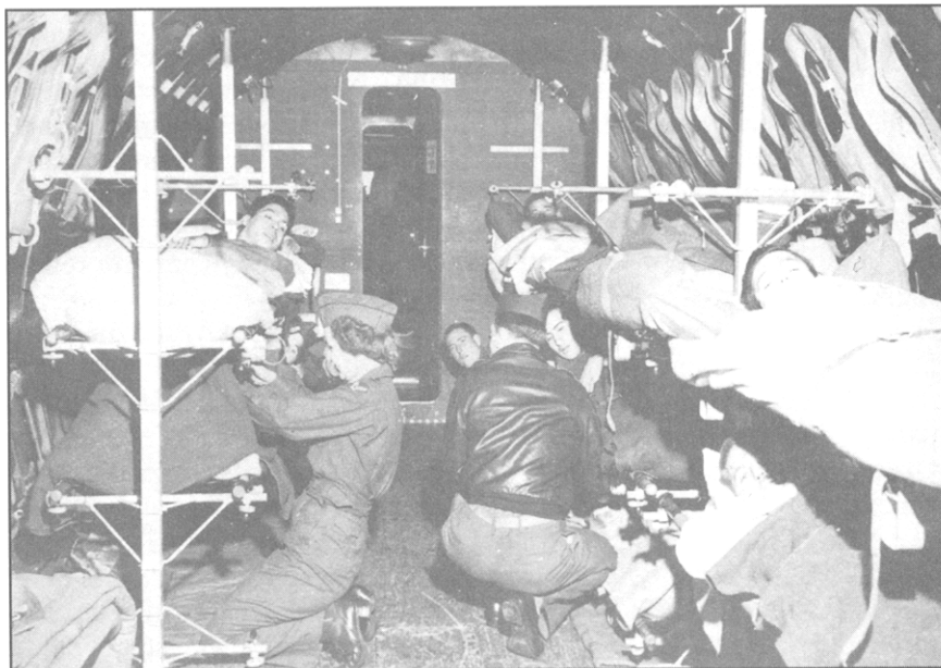
Lt. Margaret Murphy, U.S. Army flight nurse, and another member of the crew adjust traveling litters aboard an ATC C-54 Skymaster cargo plane. On return trips to the United States, the cargo craft operated exclusively as an air ambulance. Special litter supports made quartering wounded passengers swift and easy.
